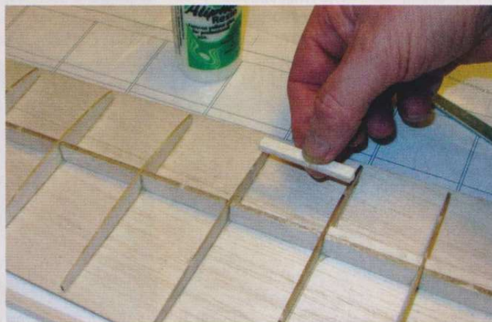
6 mm sq balsa strips were fitted 1 mm down from top of spar between ribs
