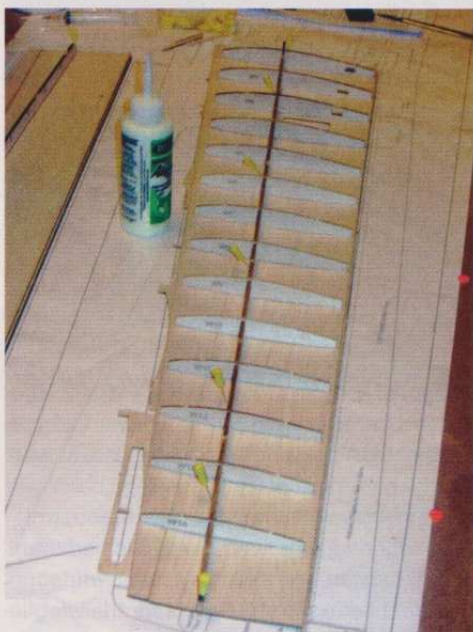
Joined balsa sheet is the base for construction of the wings, and supported with scrap wood at LE and TE while building up
