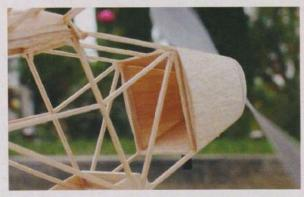
Cowl construction is clean and simple and adds a lot to the overall appearance of the model. The curved cowl "cheeks" adds very little extra weight while upping the aesthetic personality significantly. Note the "Plug-In" U.C. gusseting and structure.
