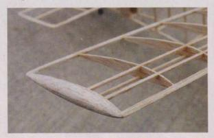
Wingtip detail shows the simplicity of the wing assembly. Strong and light will make it fly right.
