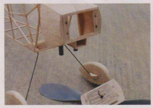
Tiny (1/16" dia. X 1/32" thick) neodium magnets aid in keeping the nose block in place during flight.
