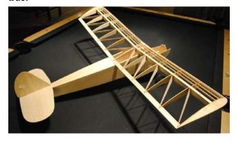
To make things even easier, our 2013 Liberty Belle is built using a laser cut wing kit and components from Stevens Aero Model and it is covered with iron-on covering film.
