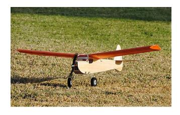
Pick a calm day and a really large space for your first flight. Do a range check and check that rudder moves freely in the correct direction. An ROG takeoff has the advantage of keeping the model safely near the ground in case it displays any bad tendencies. A short test hop might be enough to reveal any such problem.
