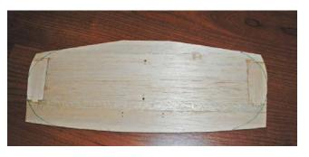
Cut out and assemble the stab. It can be made from the SA Sport Stik kit, or from scratch. Glue stab in place, aligning carefully with wing saddle.
