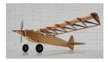
Like models today, Liberty Belle was constructed of balsa wood. The fuselage, a simple box, and the fin and stabilizer are all sheet balsa. The wing had rib and spar construction and was covered with light weight silk and painted with model airplane dope.
