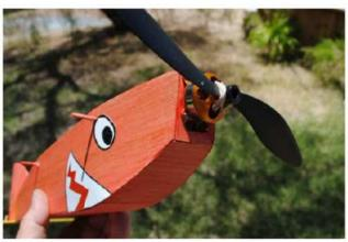
Shorten to minimum length and then solder the ESC to motor wires. Mount the motor to the firewall and attach the receiver inside the cabin with Velcro. Assemble the model with servos and battery in the fuselage. Move components for best balance and install accordingly.
