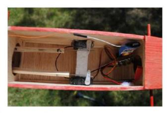
Here is a simple way to install push rods in a small model. With servos mounted and rudder and elevator installed with tape hinges, cut push rod rear exit slots in the fuselage. Cut 1/8" sq balsa push rods to length and drill a hole down the center of each end about 1/2" deep.
