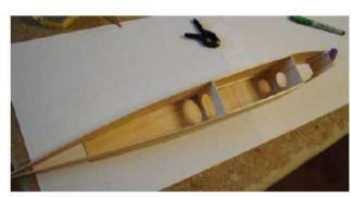
Cut stab, elevator, fin and rudder out of 1/16" balsa. Sand a bevel on mating surfaces for a hinge point. Glue stab to fuselage. Plank bottom of fuselage with 1/16" balsa forward to the first bulkhead. Plank the bottom front of fuselage with 1/32" ply.
