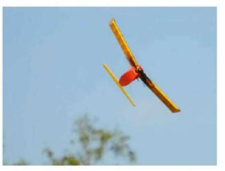
Shark-e Small RET Electric Parkflyer 22" Wingspan Wing Area 105 Sq. In. Wing Loading 6 oz. / Sq. Ft. 20 3/4" Length Weight 129g, 4 ½ Oz. Motor 2204-14T **ESC** Castle Creations Phoenix 10 Prop GWS sf 7060 Battery Nano-Tech 300mAh 2S 5.5A 6.4V 35Watts Power Flight Time About 10 Minutes Radio Hitec Eclipse 7 Berg Microstamp Servos 2 4.3g
