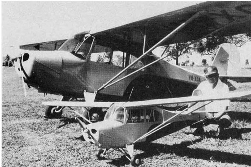
John Marquette with his 1/3 Scale Aeronca 7-AC beside the airplane he copied. Model has 11 ft. wingspan and is Tartan twin powered.
