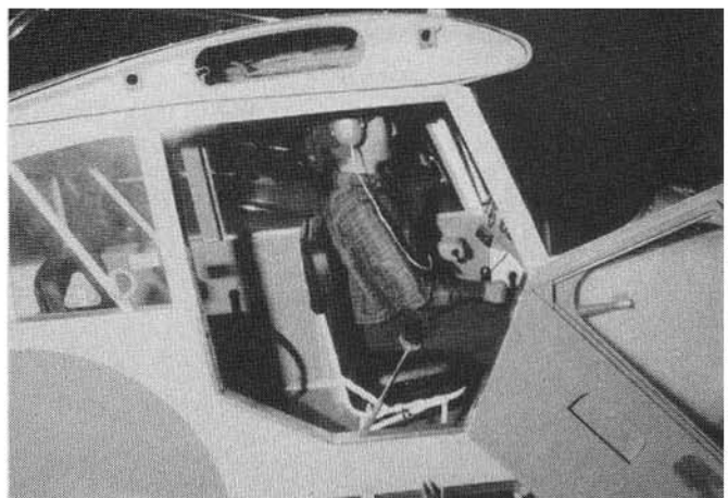
This is where the Aeronca has it all over the J-3 Cub. Cockpit room and ease of entry. Interior cockpit and door facings are vinyl.
